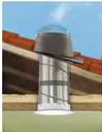
Tile flashing accessory for pitched Sun Tunnel Skylights. Engineered with a painted, malleable aluminum water diverting sheet.
